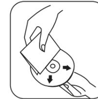
Always insert the CD with the label side facing upwards. If the CD is inserted with the printed side facing downwards, the device may be damaged.
