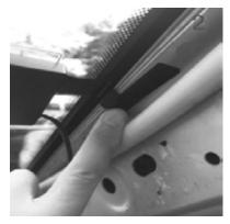
Stick the transparant part of the antenna on the windshield and put the black part on the metal frame.
