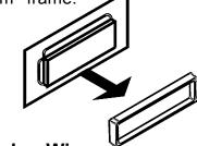
Insert the keys supplied with the old unit into both sides of the unit as shown in figure below until they click. Pull to remove the old unit from the dashboard.
