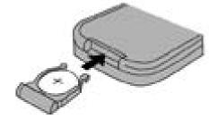
(3) Insert the battery holder into the back of the remote control.
